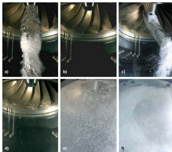
Fig 3: Typical flow patterns of a Francis turbine observed in model tests at the plant sigma: a) high load, b) around BEP, c) part load, d) low part load, e) speed no load-SNL, f) runaway speed [1].
