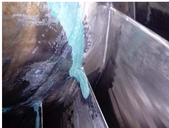
Fig 5: Detail of the strain gauge and integrated cable protection
